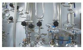
CIP&SIP, to ensure the sterility of the whole manufacturing process
