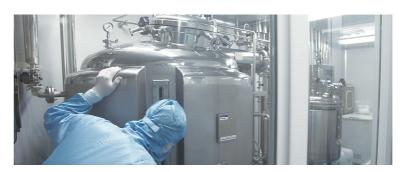
Fully automatic liquid dispensing system with the batch output of 1000 L
