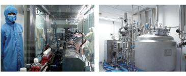
The first fully automatic liquid culture medium filling line in China Distilled water system Ensure endotoxin below 0.015 EU/ml
